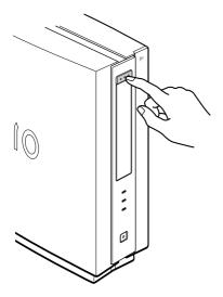
Place a CD-RW/DVD-ROM/CD-R/CD-ROM in the left-hand side of the tray with the label side facing outwards. Use the hinges to secure the disc.
